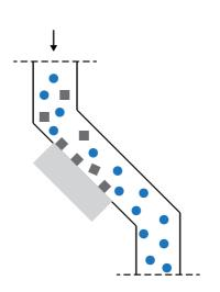
Available in two versions with ferrite or neodymium permanent magnets, magnetic plates are used primarily as protective systems for machines and other production processes. Depending on the model (ferrite or neodymium), magnetic plates can eliminate iron objects and dust of various sizes.
