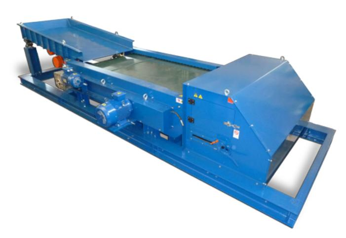
The Eddy current separator is a very efficient magnetic system for separating non ferrous metals (such as aluminum, copper, brass, etc.) from other inert materials (glass, stone, wood, etc.). This system is thus the preferred solution for many sectors such as waste management and recycling. Coupled with standard magnetic separator, ferrous metals, including that of small size, can also be separated, thus delivering optimal quality of separation.
