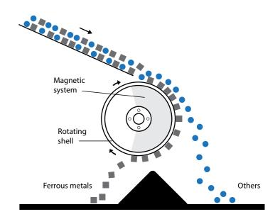
[8] Magnetic Separation [9] Magnetic Separation
